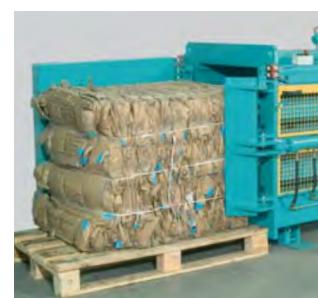
the concentrated force and the high level of automation generate a remarkable throughput performance and a high bale weight. to secure the bales there is a choice of wire or plastic tape. in combination with a tipping attachment the ideal solution for industry and warehouses.
